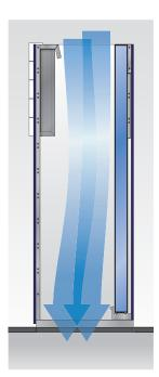
In "DX" or "CW" mode, the heat exchanger automatically moves back into position, and air-conditioning continues reliably in compressor mode or with chilled water from the outdoor chiller.
