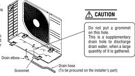
When condensed water needs to be led to a drain, etc., install the unit on a flat base (supplied separately as an optional part) or concrete blocks.
