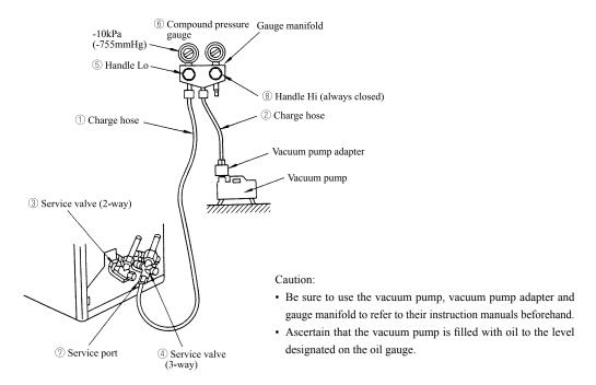
Fig.6 Configuration of air purge by vacuum pump
