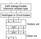
Always perform grounding system installation work with the power cord unplugged.
