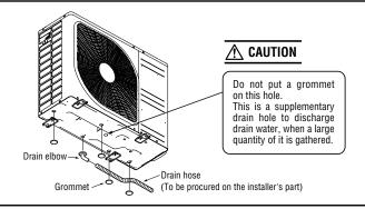
When condensed water needs to be led to a drain, etc., install the unit on a flat base (supplied separately as an optional part) or concrete blocks.
