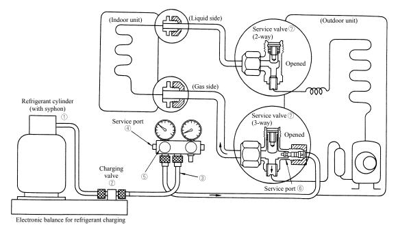
Fig.7 Configuration of additional refrigerant charging
