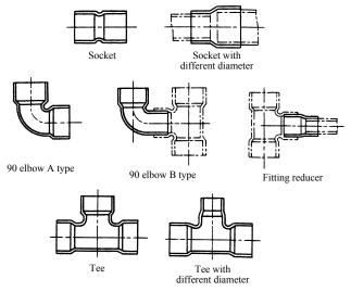
Fig.2 Socket joints
