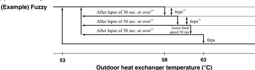
Notes (1) When the outdoor heat exchanger temperature is in the range of 58~63°C, the speed is reduced by 6 rps at each 30 seconds.
