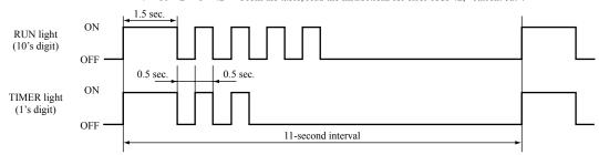
\*4: When in the service mode, when the remote controller settings (operation switching, fan speed switching, temperature setting) are set as shown in the following table and sent to the air conditioner unit, the unit switches to display of service data.
