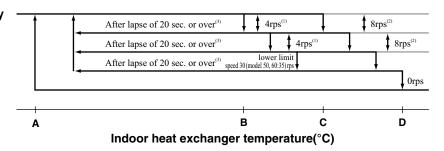
Notes (1) When the indoor heat exchanger temperature is in the range of B~C °C, the speed is reduced by 4 rps at each 20 seconds.
