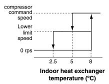
Notes (1) When the indoor heat exchanger temperature is in the range of 2.5~5°C, the speed is reduced by 4 rps at each 20 seconds.
