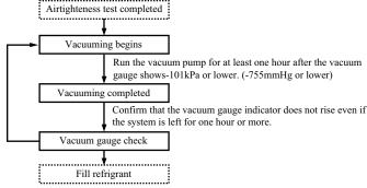
When the system has remaining moisture inside or leaky point, the vacuum gauge indicator will rise.
