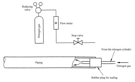
Fig.5 Prevention of oxidation during brazing
