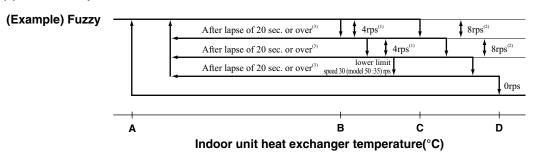
Notes (1) When the indoor heat exchanger temperature is in the range of B~C °C, the speed is reduced by 4 rps at each 20 seconds.
