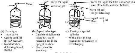
Fig.8 Cylinder types
