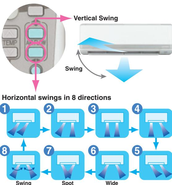
The airflow direction from the right and left louvers can be controlled individually. Eight different air flow patterns can be selected.
