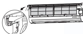
When removing the air inlet panel for internal cleaning or others, open the grill and then pull it to this side.
