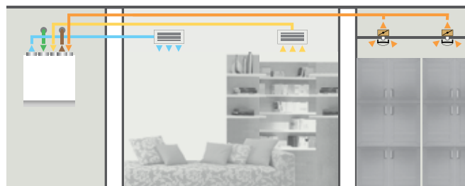
With separately connected additional extract air diffusers If a kitchen hood is not used, an extraction diffuser from the bathroom, laundry, or other premise can be connected to the unit as well.
