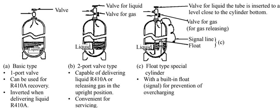
Fig.8 Cylinder types
