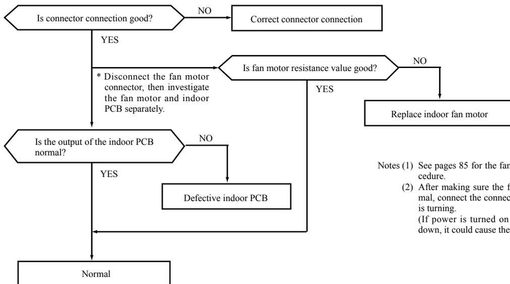
Notes (1) See pages 85 for the fan motor and indoor PCB check procedure.
