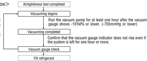
When the system has remaining moisture inside or a leaky point, the vacuum gauge indicator will rise. Check the system for a leaky point and then draw air to create a vacuum again.
