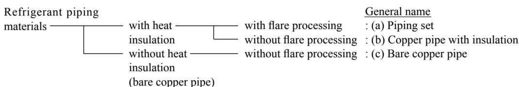
As R410A features pressure about 1.6 times higher than R22, it is necessary to use a copper pipe which has a thickness stated in Table 3 (see page 92) and which contains less contaminants. It is necessary to carefully treat/store copper pipes so that they are not collapsed, deformed or damaged. Due care must also be exercised so that foreign matters such as dust and water do not enter the pipe interior.
