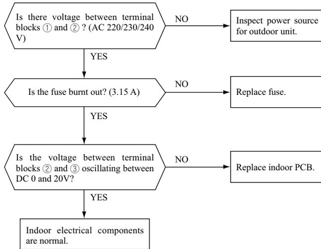
**(b) Indoor unit fan motor check procedure**
