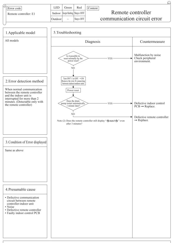
Note: If the indoor unit cannot communicate normally with the remote controller for 180 seconds, the indoor contnrol PCB starts to reset automatically.
