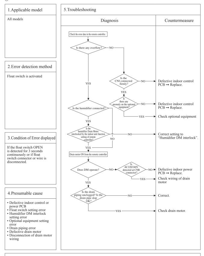
Note: When this error occurred at power ON, disconnection of wire or connector of the float switch is suspected. Check and correct it (or replace it, if necessary).
