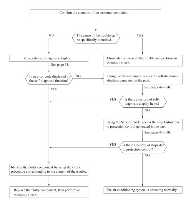
Note (1) Even in cases where only intermittent stop data are generated, the air conditioning system is normal. However, if the same protective operation recurs repeatedly (3 or more times), it will lead to customer complaints. Judge the conditions in comparison with the contents of the complaints.
