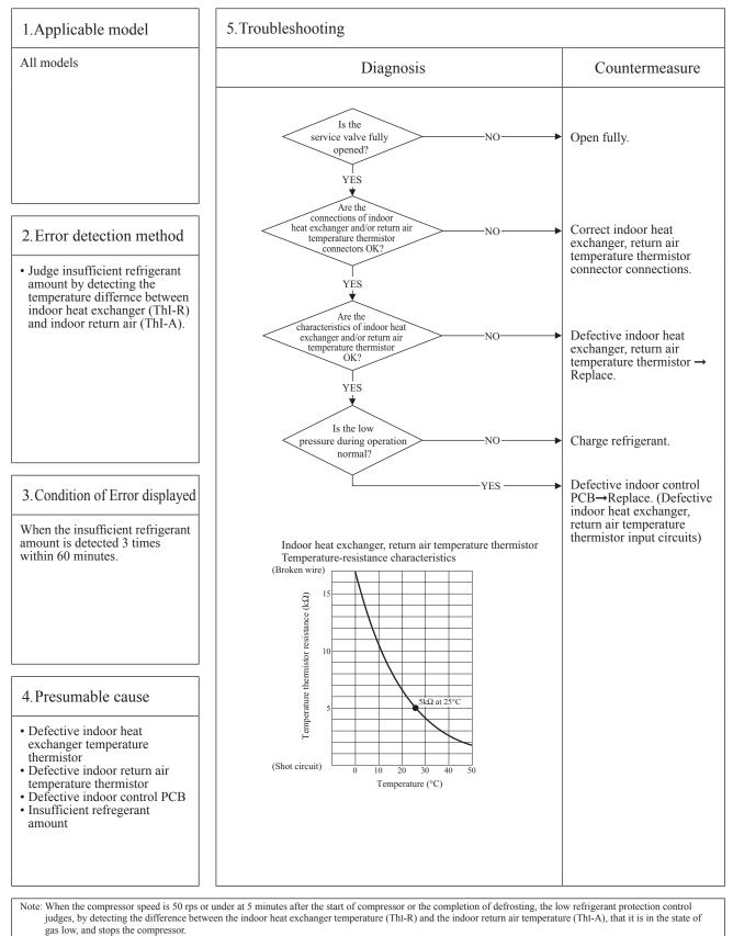
Cooling: Indoor return air temperature (ThI-A) – Indoor heat exchanger temperature (ThI-R)  $\ge$  4 deg Heating: Indoor heat exchanger temperature (ThI-R) – Indoor return air temperature (ThI-A)  $\le$  6 deg
