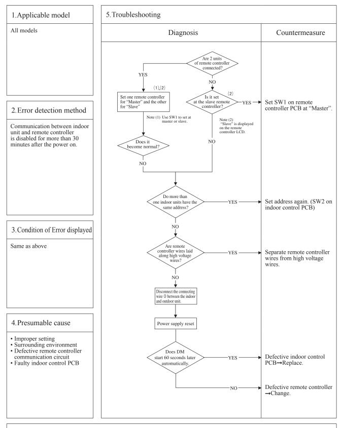
Note: If any error is detected 30 minutes after displaying "OWAITO" on the remote controller, the display changes to "INSPECT I/U".
