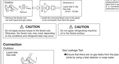
OConnect the pipes on both liquid and gas sides
