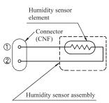
Remark: Do not perform a continuity check of the humidity sensor with a tester. If DC current is applied, it could damage the sensor.
