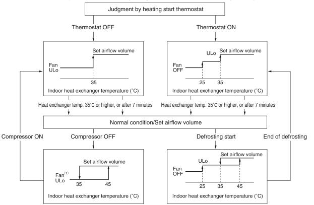
Note (1) Heating preparation is displayed during the hot start (when the compressor is operating and the indoor fan does not provide the set airflow volume).
