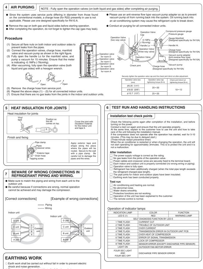
The connection of the earth cable to the following substances causes dangerous failures, therefore it shall never be done. (City water pipe, Town gas pipe, TV antenna, lightning conductor, telephoneline, etc.)
