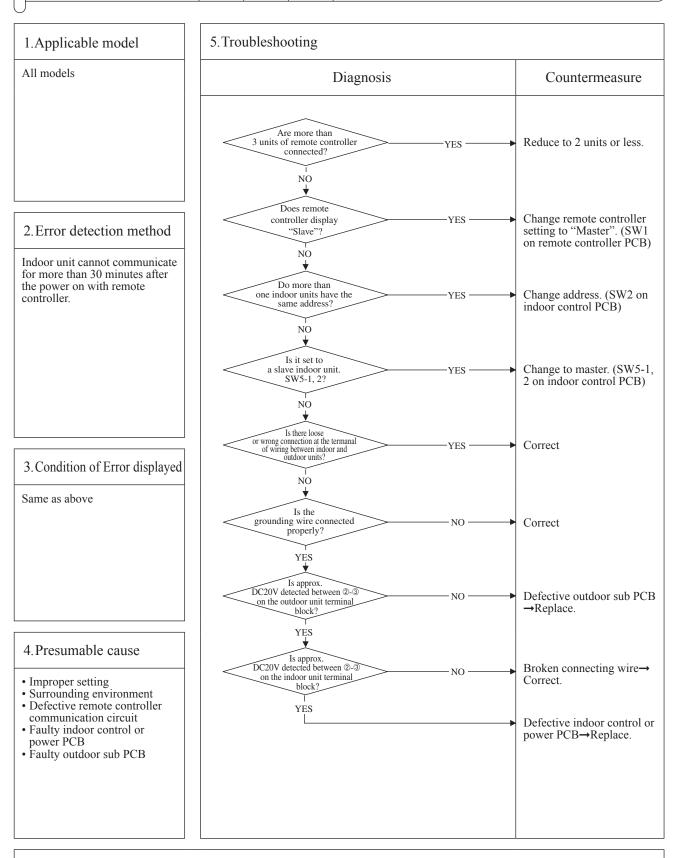
Note: If any error is detected 30 minutes after displaying ""WAIT"" on the remote controller, the display changes to "INSPECT I/U".
