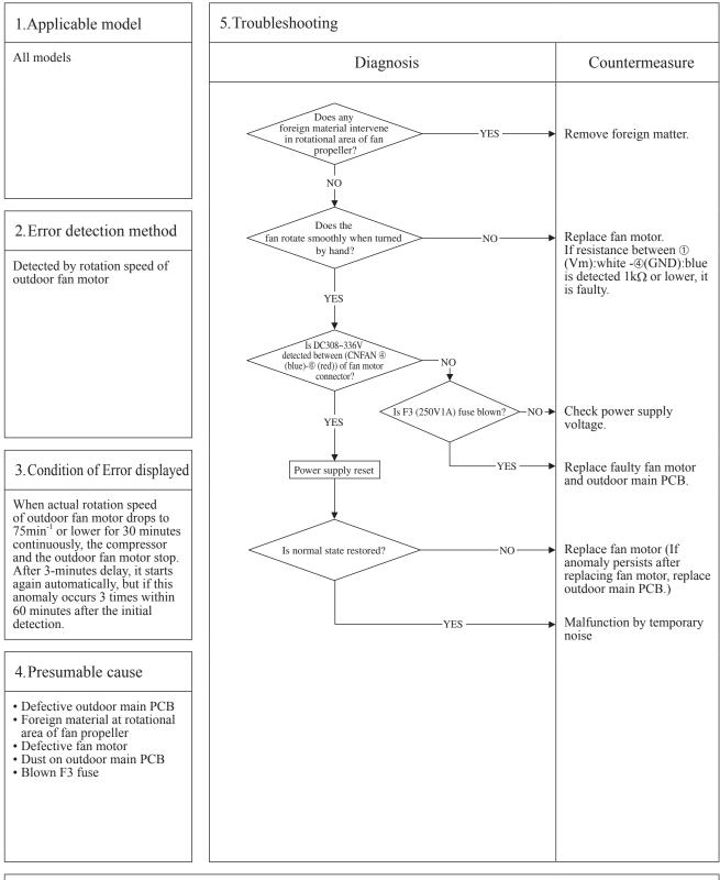
Note: When E48 error occurs, in almost cases F3 fuse (1A) on the outdoor main PCB is blown. There are a lot of cases that fuse is blown and E48 occurs due to defective fan motor. And even though only the outdoor main PCB (or fuse) is replaced,, another trouble could occur. Therefore when fuse is blown, check whether the fan motor is OK or not. After confirming the fan motor normal, check by power ON. (Don't power ON without confirming the fan motor normal.)
