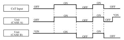
Note (1) The ON with the \* mark indicates an ON operation using the remote control unit switch, etc.
