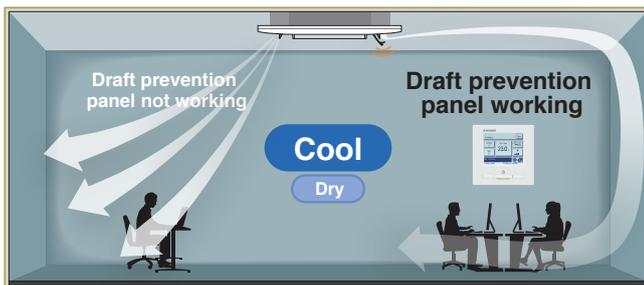
User can position panels by using the remote controller only (RC-EX3A, RCN-TC-5AW-E2, -E3) when Draft Prevention Panel is available.
